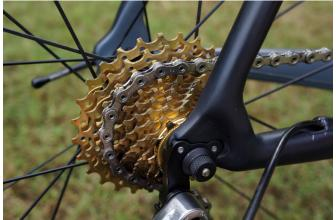
Compared to a steel cassette the weight savings are substantial. The cassette pictured is only 161 grams, whereas an OEM Shimano 105 12 thru 25 cassette is 252 grams – equivalent to the weight of 20 Canadian Quarters.
