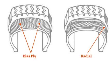
In the bias-ply tire the cords tend to rub against each other and that means greater rolling resistance. That friction is dissipated as heat. On bicycle tires internally produced heat isn't a big concern.
