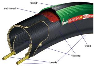
Bicycle tire construction is very much like that of automotive, heavy duty/off-road or aircraft tires – just smaller. Although radial-ply designs have been marketed, their cost and feel have made them a nonstarter for the bicycle market. So, almost 100% of bicycle tires are bias-ply designs, even though bias-ply designs do offer more rolling resistance than radial-ply designs – bias-ply is king.
