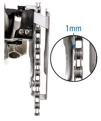
If you cannot get the derailleur to latch and the shifter requires a lot of effort, it likely means that the high limit screw is set too tight and the brifter is unable to reach the high latch point. Back off the "H" screw a quarter turn and recheck if the derailleur will latch in the high position. Keep backing off the screw until you can get the derailleur to latch in the high position. Cable tension may need to be increased as well.
