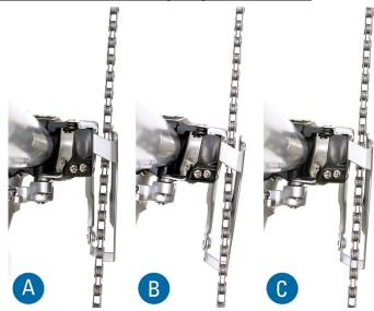
3. The low limit is set first by adjusting the screw marked "L" until there is minimal clearance (1 mm) between the chain and the inner derailleur cage (below). Not all chainrings are true, so be sure to rotate the crankset to ensure that all areas of the chainring rotate without rubbing.
