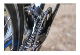
Remount the chain onto the small chainring and again upshift all the way to your high position. Is the chain rubbing on the outside of the derailleur cage? If so, you need to turn the "H" screw out and perhaps add some cable tension to get the derailleur to a point where rubbing stops. Now to check if you have 4 distinct detent points (with trim).
