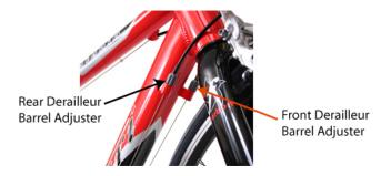
So now the question becomes which way do I turn it? As a reference, a properly tuned rear derailleur will shift the chain one cog for every half revolution of the crankset.
