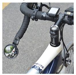
Many of these mirrors are poorly designed with insufficient damping of the mirror. The result is that it can be difficult to clearly see detail, such as whether-or-not the driver approaching from the rear has noticed you.
